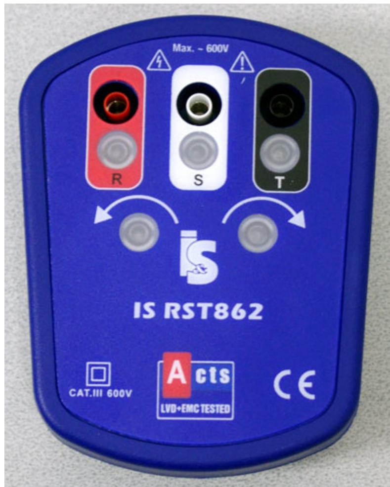
**IS RST862 MISURATORE DEL SENSO CICLICO DELLE FASI**
